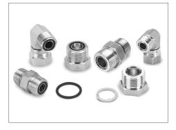
**Robust Port Stud™** – Features a longer locknut to cover the uppermost threads on SAE adjustable port end fittings, eliminating the potential for backup washer damage and leaks.
